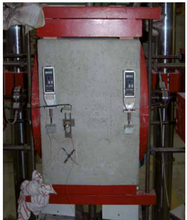
Test setup for cyclic load test
