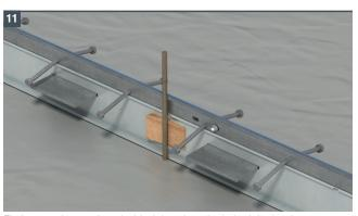
Fit the wooden wedges behind the pin to lock the joint in place.
