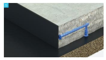
If specified apply expansion material to the slab face.
