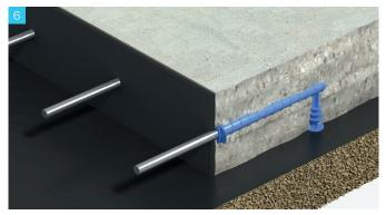
insert the appropriate dowels into the sleeves as the next pour is being prepared. To eliminate tripping, the dowels can be installed after the groundwork has been completed for the adjacent pour.
