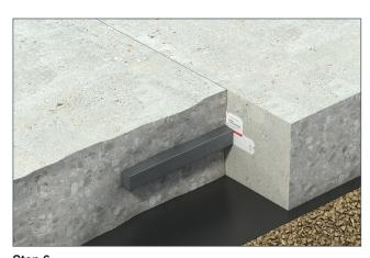
**Step 6**Once dowels have been correctly positioned, install the specified reinforcement and carry out the next pour. For expansion joints, install compressible material before second pour.
