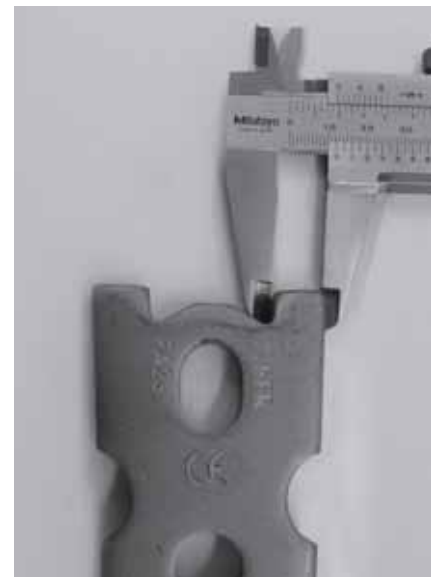
Checking the dimensions of a HALFEN FRIMEDA TPA Anchor
