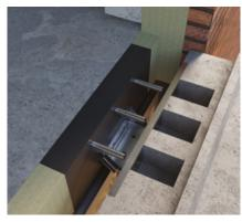
For fixing from the balcony side, recesses are formed in the balcony, allowing for connection from outside the building. In some cases the facade can also be installed before connecting the balconies.
