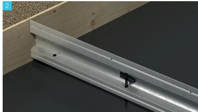
Adjust the key joint to the correct height and secure by tapping in the supplied wedges. If capping strips are to be used allow the appropriate set down distance and apply capping strip prior to pouring concrete.
