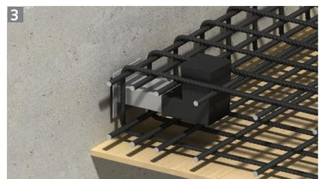
Puncture the label of the sleeve to reveal the cylindrical sleeve only. Push the sleeve over the dowel until it is flush with the concrete. Tie sleeve to reinforcement and pour concrete. See steps 4 to 6 above to complete installation.
