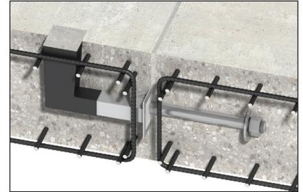
*The Lockable Dowel accommodates initial concrete shrinkage and is then locked in position with a mechanical plate and epoxy resin.*
