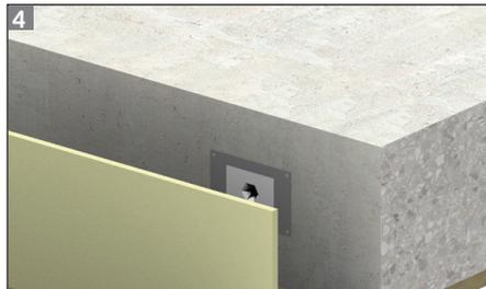
4 Position the compressible joint filler of the appropriate width for applications where movement is expected between the two sections of concrete.
