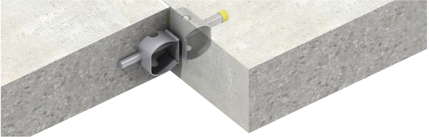
The HALFEN HSD-ULTRA is a shear dowel system for high loads. The steel plates in the area around the dowel and the sleeve distribute the load in the concrete and allow higher loads than conventional shear dowels.
