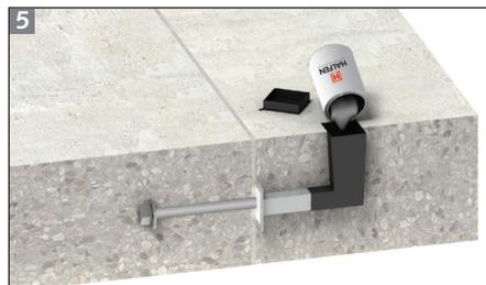
Mix the two-part epoxy resin and pour into the void former. It is essential the resin flows along the stainless steel box section towards the joint and reaches the notches on the locking plate, which indicate minimum resin depth.
