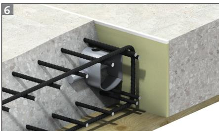
6 Fix the local reinforcement in position around the dowel component together with any other reinforcement that is required, ensuring that the correct cover to the reinforcement is maintained. Pour the concrete to complete the installation of the shear connector.
