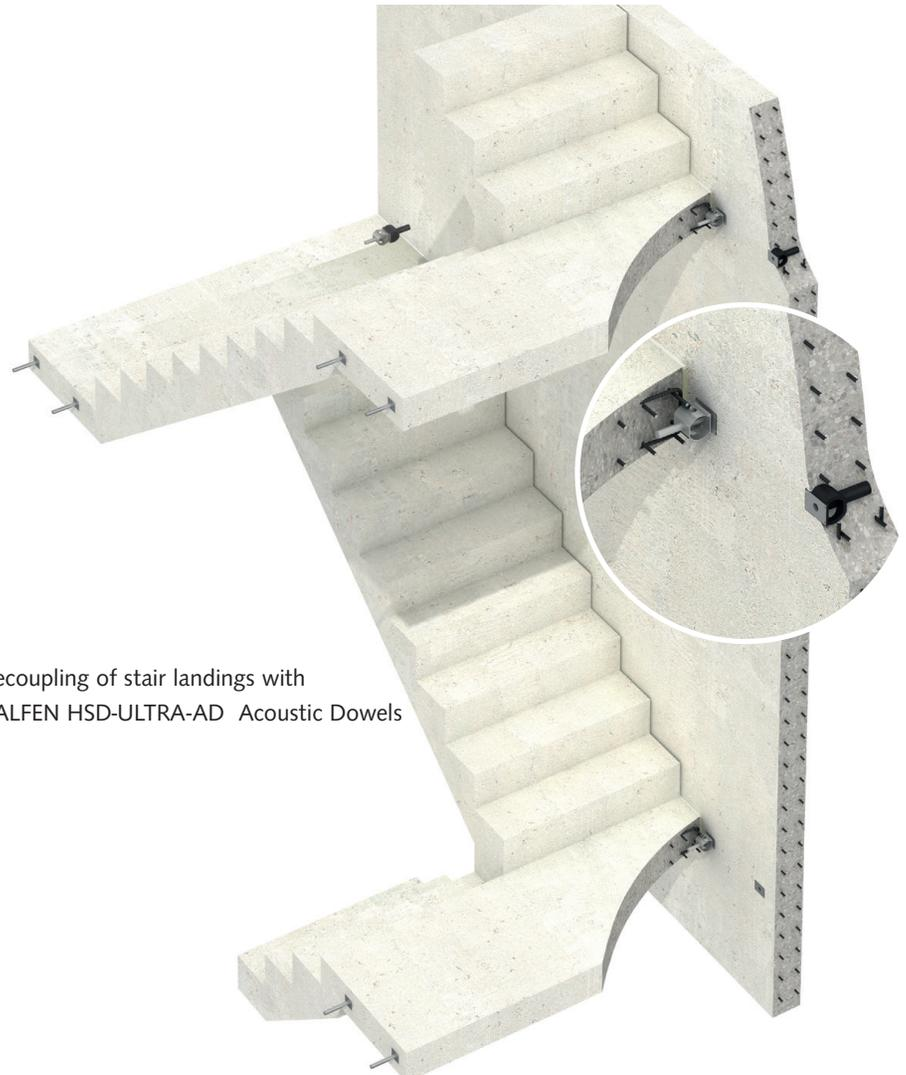
Decoupling of stair landings with HALFEN HSD-ULTRA-AD Acoustic Dowels
