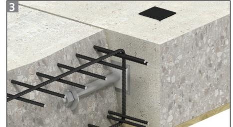
Place the local reinforcement around the dowel component and pour the concrete.
