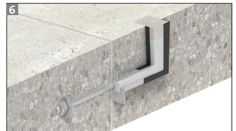
After 24 hours the void former can be filled with cementitious material, level with the top of the slab, to complete the installation. The locked dowel continues to transfer vertical load between the slabs, but movement can no longer take place.
