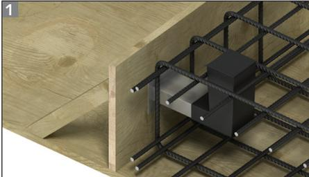
Nail the sleeve to the formwork either central in the slab or for slab depths over 12" so the top of the void former is level with the top of the slab. Do not remove the label over the nailing plate as this prevents ingress of concrete into the sleeve. Place the local reinforcement, as specified on engineer's drawings.
