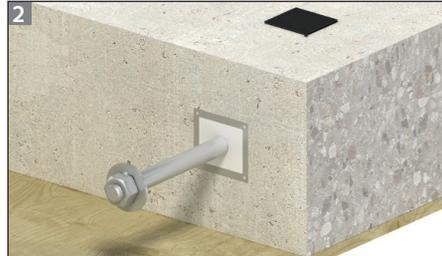
Pour the concrete, and when the required strength is attained, remove the formwork. Puncture the label to reveal the cylindrical sleeve only and insert the dowel until it is approximately  $\frac{3}{4}$ " from the back of the void former.
