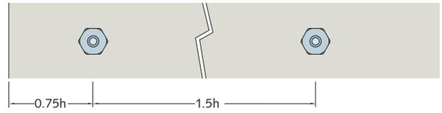
HSD-LD-20W Minimum Edge Distance and Spacings. h = depth of adjoining slab
