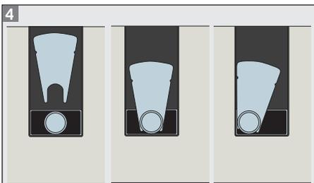
After a predetermined time period (generally 28-120 days), when movement between the slabs has stabilized, the dowel is ready to be locked. Fit the Locking Plate on a groove in the center of the void former. The fan-shaped Locking Plate allows the dowel to be locked in any position.
