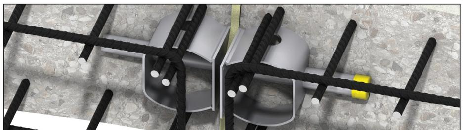
Notes: (i) Although installation is shown for HALFEN HSD-ULTRA, the procedure is the same for all HALFEN HSD Shear Dowels.
