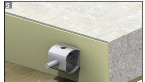
5 Push the dowel component through the joint filler (if applicable) until it is fully located in the sleeve component. It may be necessary to tap the dowel component to overcome the dimple which pinch holds the dowel in the sleeve and prevents dislocation when the concrete is vibrated.
