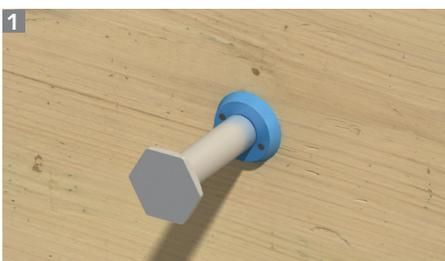
Nail the threaded anchor to the formwork so the dowel will be central in the adjoining slab or within 6" of the top of slabs over 12". Place the local reinforcement as specified on engineer's drawings and cast the concrete.
