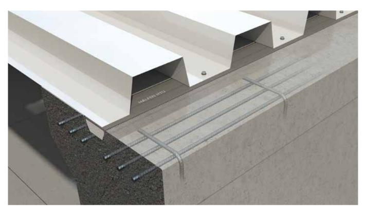
The HALFEN HTU Channels are ideal for simple fixing of all types of profiled metal sheets or sandwich panels – using self-tapping screws. Thanks to its innovative shape and profiling, the new, optimized generation of channels are self-anchoring and are cast completely into the concrete cover.
