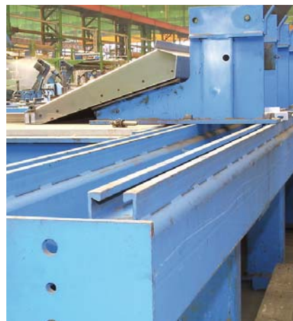
Welding-jig, locomotive construction
