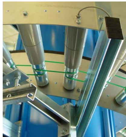
Cantilever fixing on a vertical conveyor system
