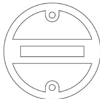
The CP-2 Coil Setting Plug – Plastic is available in  $\frac{1}{2}$ ",  $\frac{3}{4}$ " and 1" diameters. They are effectively used to set inserts in the form by nailing the plug to the form face and then threading the coil insert onto the plug. The reusable plugs are easily removed from the concrete after the form has been stripped. The Coil Setting Plug can also be used as a temporary cap when another pour will be made at a later time.
