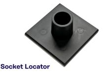
The SPSL-1 manhole step socket locator helps secure proper placement of the manhole step socket prior to concrete pouring
