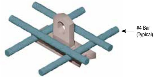
Typical method of reinforcing Plate Anchors
